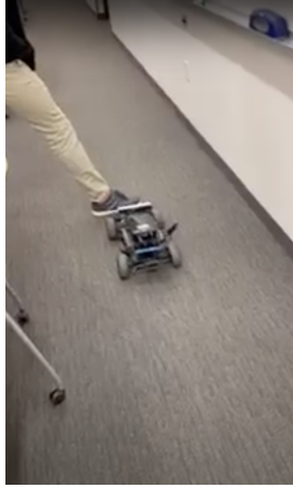
Figure 5: Our teammate placed his foot in front of the racecar while it was executing the wall follower to test our safety controller performance. The racecar successfully stopped in front of our teammate's foot.
