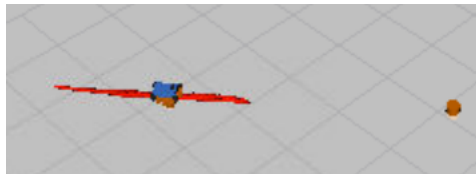
Figure 8: Racecar simulator in Rviz demonstrating both motion model and sensor model on and deterministic set to False. The particles very closely followed the racecar, and can be seen as the orange clump under the racecar.
